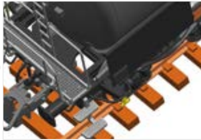
Shunter's platform and walkway grids of open design
