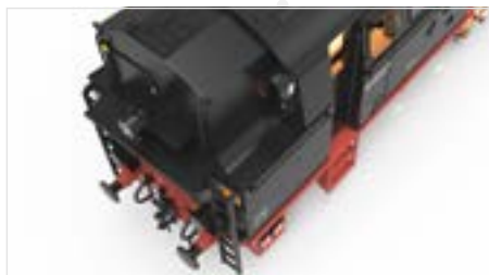
Free-standing top headlight and separately applied handrails and ladders
