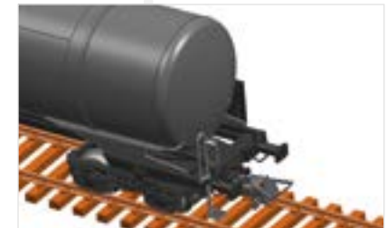
Free-standing handrails and shunting tread
